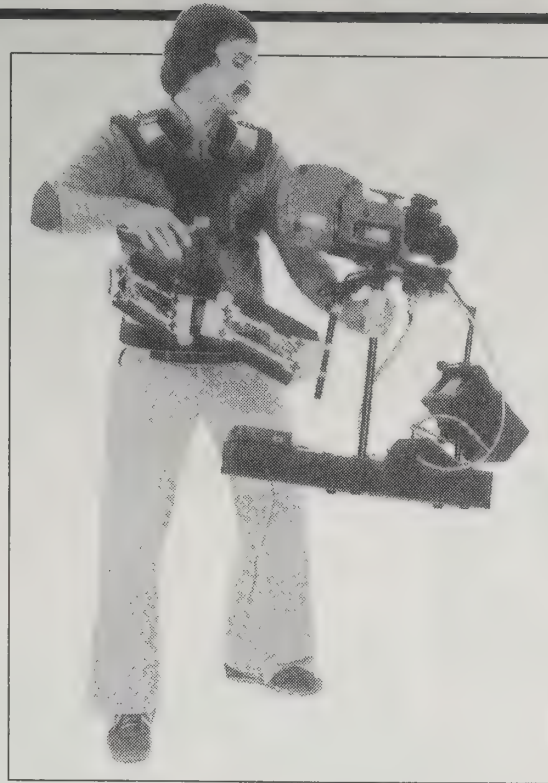
The Steadicam. Expensive and cumbersome, it is the last word in smooth hand-held cinematography, and has been used to good effect on many features. (Cinema Products)
